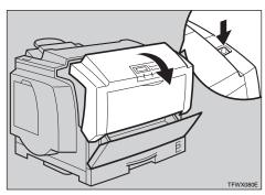
Holding the green inset grips of the photoconductor unit, pull the top of the unit forward.
